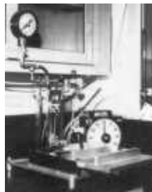
Figure 34. Pouch air burst tester.
